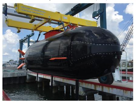
Dry Combat Submersible undergoing sea trials and testing in open waters. Photo: Msubs (source)
