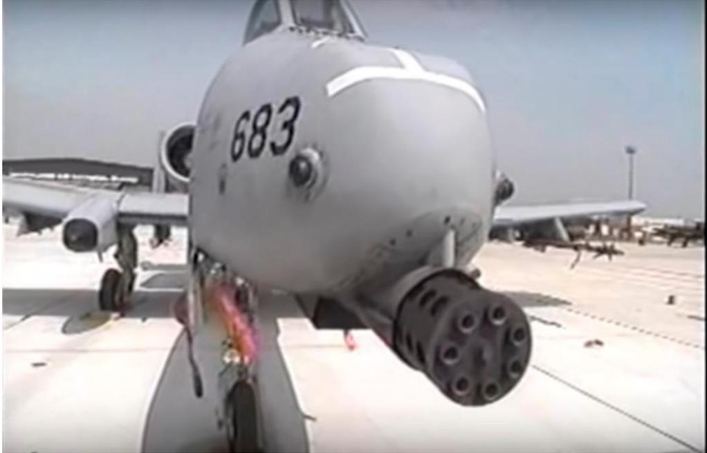
Figure 2. The A10 Warthog 30 mm Gatling gun fires DU rounds.
