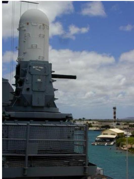
Figure 3. Depleted Uranium Gatling gun radar assembly on the USS Missouri, Pearl Harbor, Hawaii, for interception of oncoming missiles and attacking fast boats. Photo: M. Ragheb.
