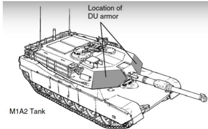
Figure 1. The USA Abrams M1A1 tank uses depleted uranium shields at the front of the turret and boron ceramic armor plates and fires depleted uranium munitions. High carbon steel and composite boron ceramic act as shield against radiation. Source: USA Army.
