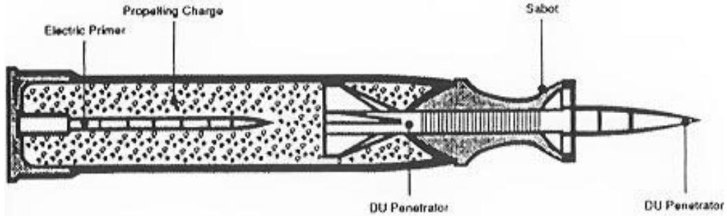
Figure 7. Schematics of a sabot armor piercing rounds with a depleted uranium penetrator.
