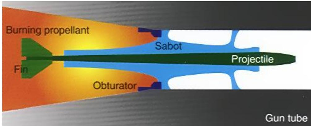
Figure 9. Cross Section of sabot showing kinetic energy transfer from the propellant to the sabot.
